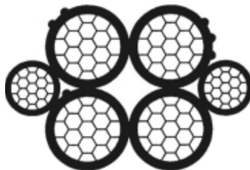
Insulated 4 bundle configuration with two additional cables of a smaller cross section
