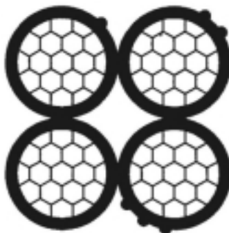
Insulated 4 bundle configuration
